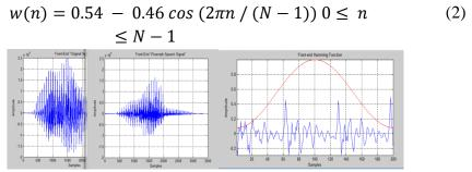
Figure 2: Original signal, pre-emphasis, and Hamming Window
